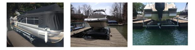
3. A **Refurbished HydroHoist Lift** is yet another option available for getting your boat out of the water. It is a lift built with all new components except the tanks. The tanks have been washed, checked for leaks, and painted with the best paint available for this application. The lift will be built with brand new components which means the first major maintenance should be around 17-19 years after installation. Refurbished lifts are subject to availability.
